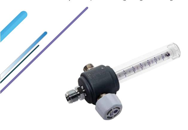
The measuring unit (graduated rod and graduated rod cover) is made of polycarbonate, a material with high mechanical resistance which therefore makes this device particularly suitable for the heaviest uses. The use is simple. just connect the device to a centralized hospital system through the specific gas and norm connector (outlet). Once engaged, the flow delivered is regulated by the front adjustment tap, with micrometric pitch for a more precise adjustment.
